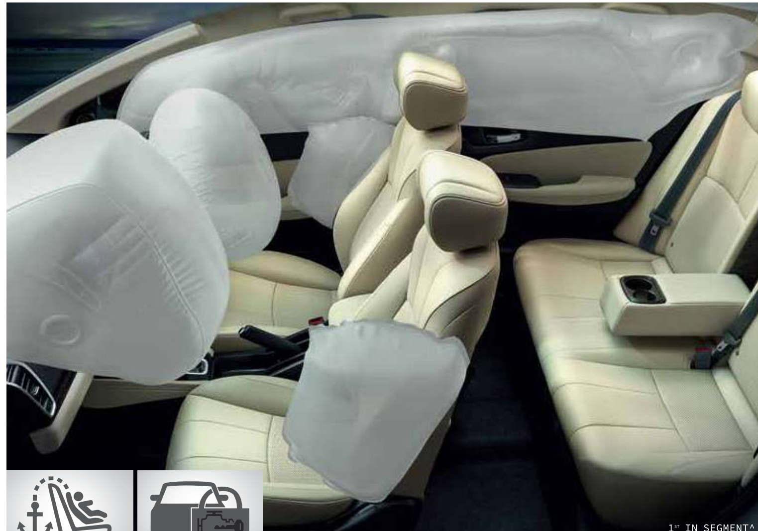
6 AIRBAGS SYSTEM (DUAL FRONT i-SRS ^ AIRBAGS, FRONT SEATS i-SIDE AIRBAGS & SIDE CURTAIN AIRBAGS)
